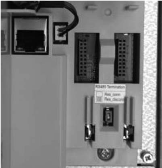
Figure 36. RS-485 bus termination setup
