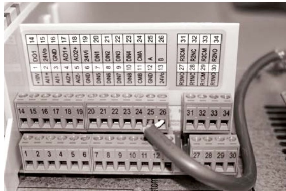
Figure 63. Connection of SmartWire-DT module with PowerXL DG1 Drive
