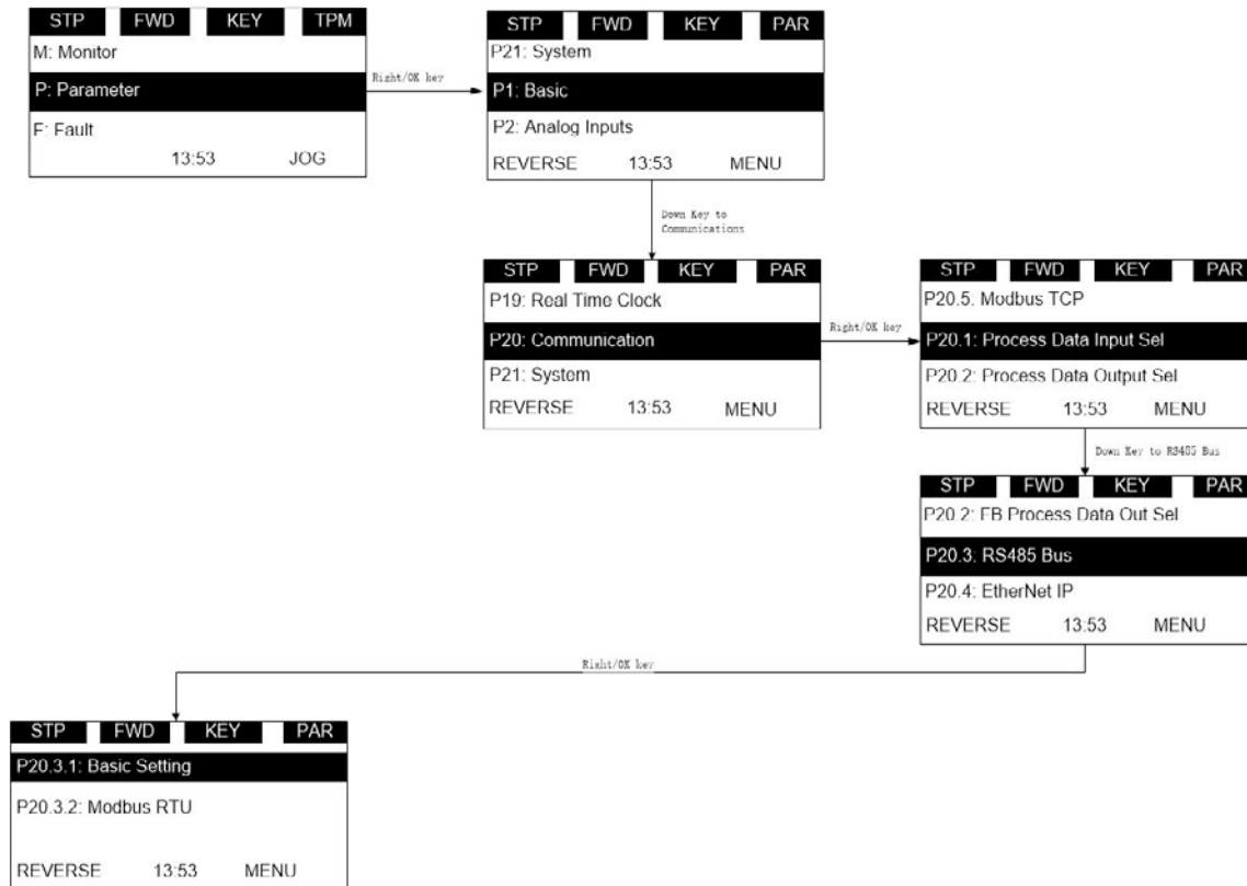
Figure 38. PowerXL DG1 BACnet MSTP parameter navigation
