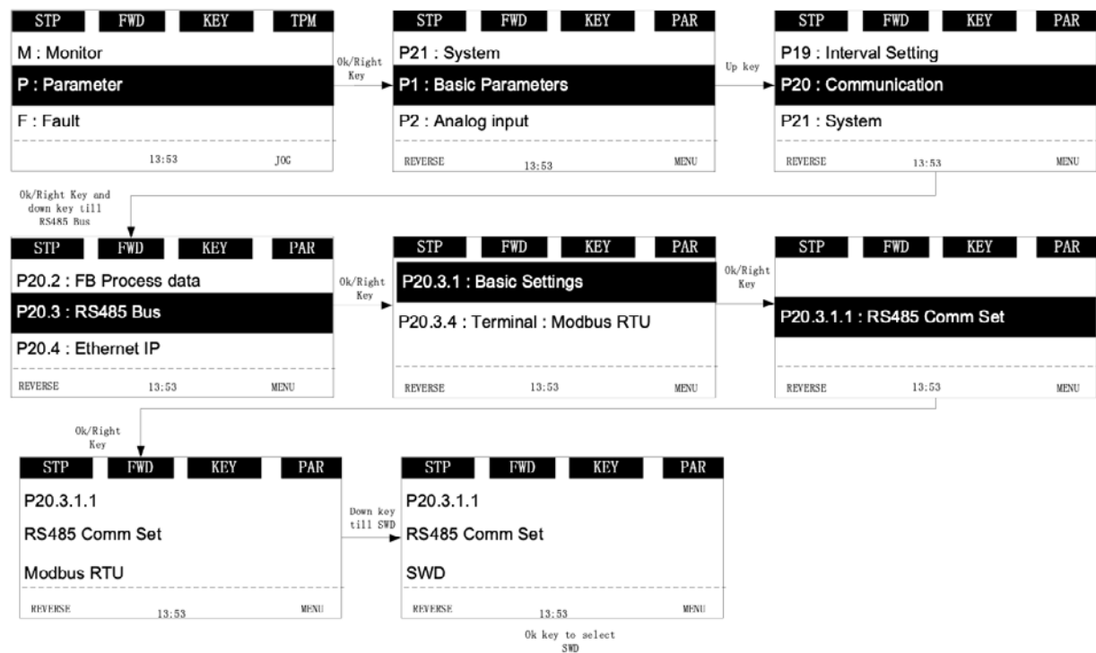
Figure 65. DG1 keypad navigation to enable SmartWire-DT
