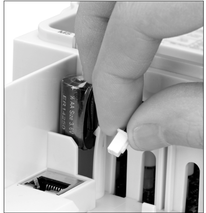
Figure 1. RTC battery connection
